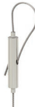
"The Pushmepullyu" Quick Loopmaker DG-15ZZ Maximum allowable weight: 80lbs w/ 1/16"(1.6mm) cable, 40lbs w/ 3/64"(1.2mm) cable.
