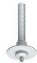
Acoustic Tile Drywall Gripper DG-12-CPLT-SAT Connects to ceiling tile or drywall. Excess cable passes through the hollow thread. For 1/32" - 3/64" cable only. Comes w/ toggle nut. Maximum weight 5 lbs. pg. 6
