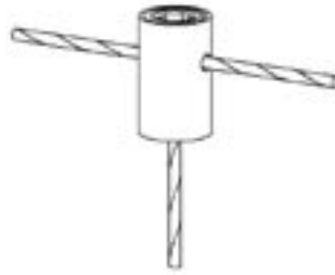
CC-M8-Q2.9 Cross-Cable connector
