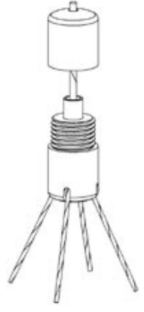
15-SPT4 Sputnik assembly for 3/64" and 1/16" cable
