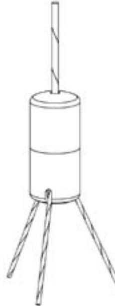
15-SPT3 Sputnik assembly for 3/64" and 1/16" cable
