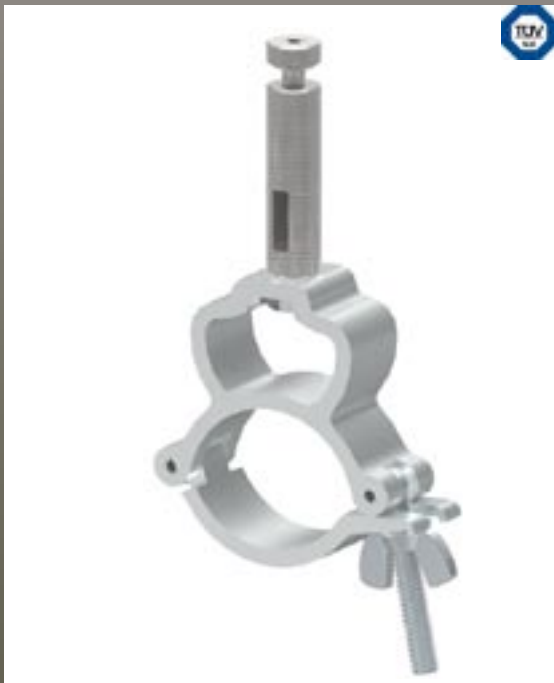
30Z-CLMP-200-V6 Side Exit Gripper with Clamp Attachment, 6-Ball Mechanism, For Pipe or Truss from 1.25" - 2.0" OD, Safety Nut
