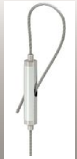
ZF-30ZZ Double Ended Loopmaker Gripper, 3-Ball Mechanism SWL: 250 LBS
